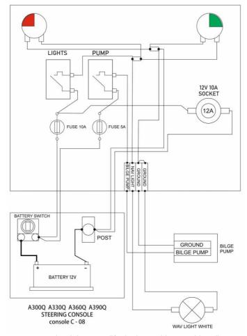
The manufacturer reserves the right to modify the boat wiring or wiring diagram without notice.
